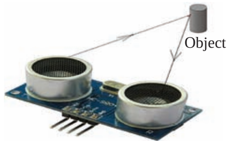
Figure 4.16 : How an ultrasonic sensor works
