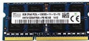
Figure 1.12 : Random Access Memory (RAM) card act as the main memory
